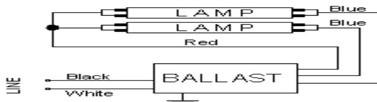
Note: For one lamp application, cap any blue lead. Insulate to 600 volts.
